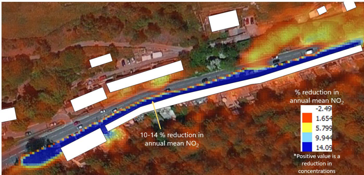
Figure 31: Visualisation of difference in modelled concentrations of NO 2 for 2017- Scenario 15
